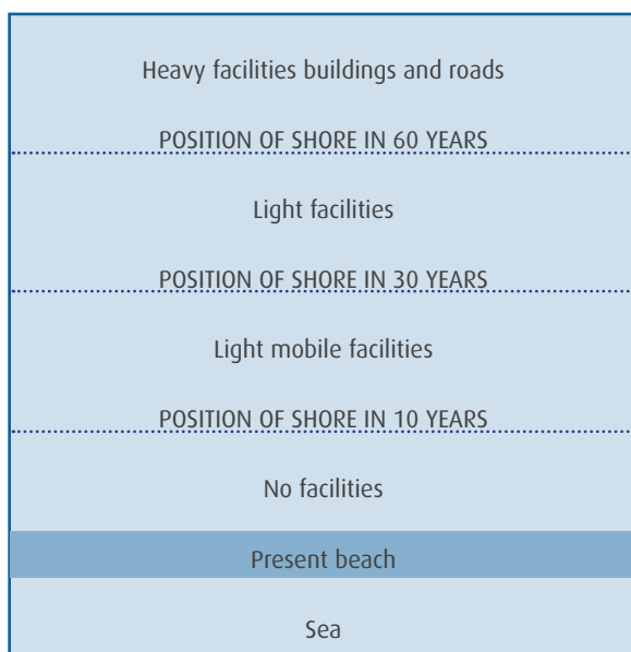
Figure 1. Propositions for rational management of coastal areas in a situation where the shore line retreats (according to Cazes-Duvat and Paskoff, 2004 18 )
