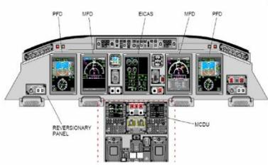
The **PRIMARY FLIGHT DISPLAY (PFD)** displays information such as airspeed indicator, altitude indicator, ADI, IRS, vertical speed indicator, radio aids, autopilot, flight director and radio altitude data. They are displayed in two sections, top and bottom, each one presenting a group of information.
