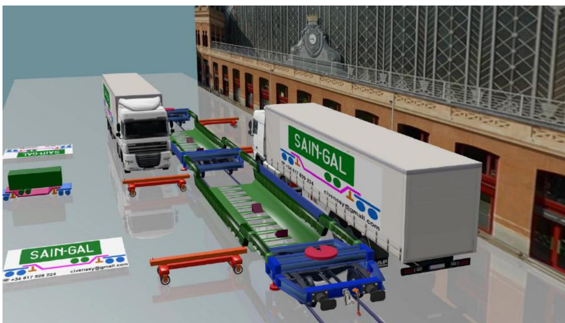
Figure 1-3. Sain-berceau en position.
