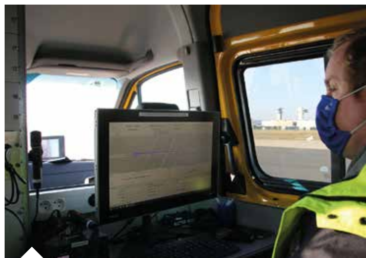
ATSEP measuring the ILS signal on the runway axis at Paris-Orly airport (regulatory check).
