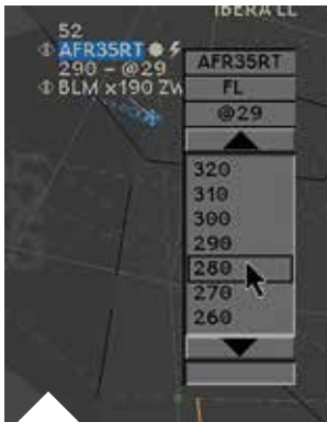
Reims ACC: level clearance (FL) given by the controller via Data Link, symbolised by the lightning flash next to the AFR call sign.
