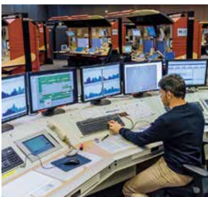
The Flow Management Position in ACC has tools with very advanced functionality for fine-tuned management. It optimizes the capacity of the airspace in collaboration with the European Network Manager (EUROCONTROL).
