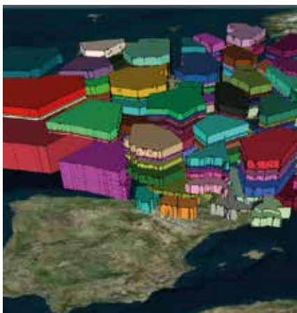
France's airspace comprises 168 basic sectors, which may be optimised depending on the traffic characteristics.
