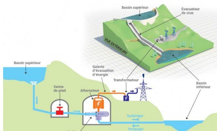
Figure 1 Operating principle of a PSH plant - Source EDF
