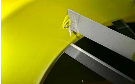
Photographs : plastic on the fenestron and the nacelle, and an identified piece
