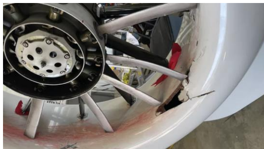
Photographs: damage to the fenestron
